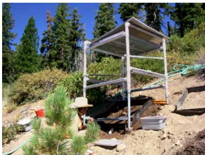
Rainfall simulation is a tool that is used to simulate rainstorms and directly measure surface erosion and infiltration rates.
