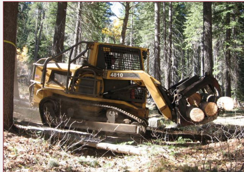
Skid steer loader transporting logs across a Humboldt crossing.
