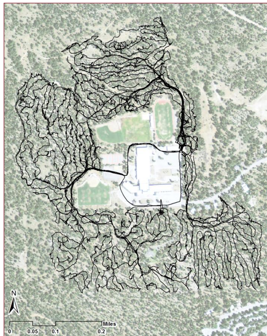
Figure 25. Cut-to-length equipment travelways mapped using a GPS unit. Large numbers of passes were concentrated along a few main trunk lines.
