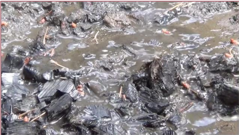
Turbid water running off surface of unmitigated burn scar during runoff simulation.
