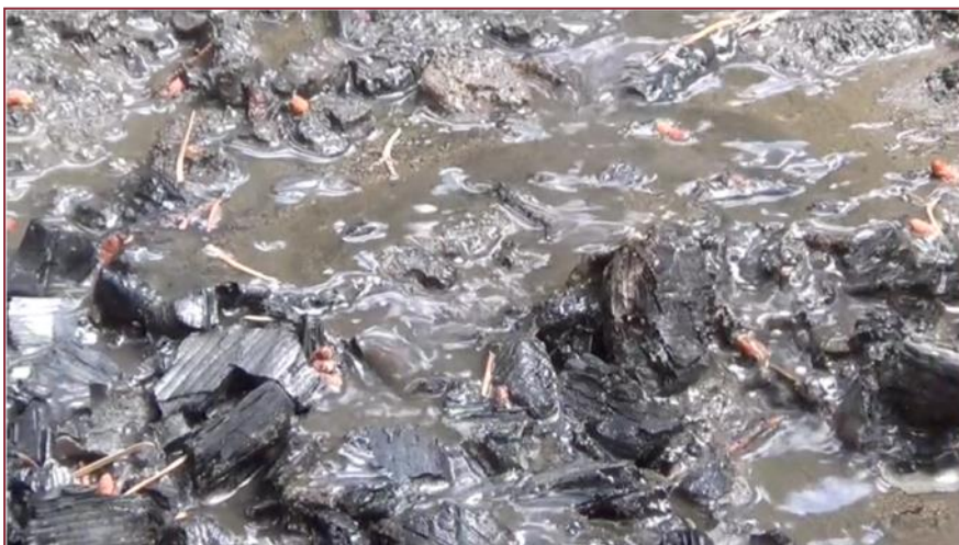
Turbid water running off unmitigated burn pile during runoff simulation.
