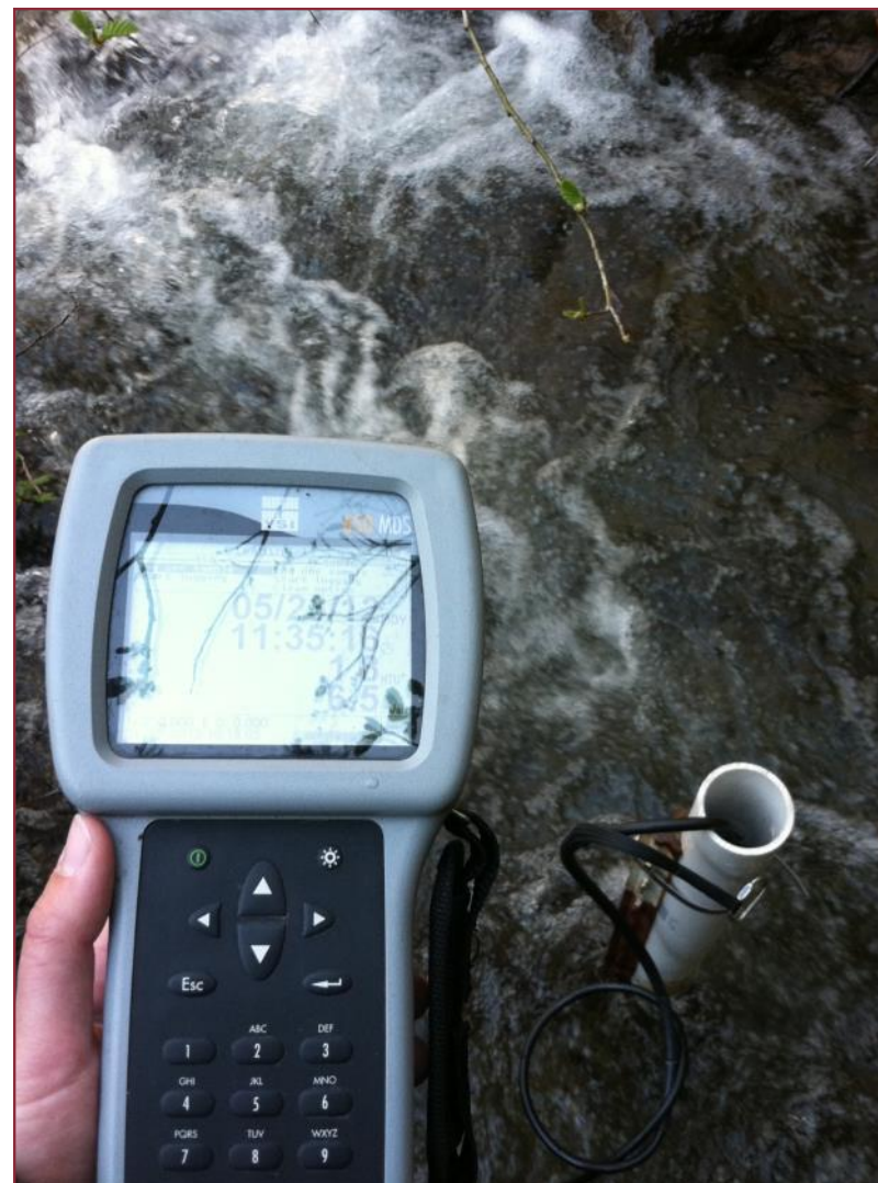
Using a multi-parameter data logger to upload 15-minute turbidity data from a turbidity sensor.
