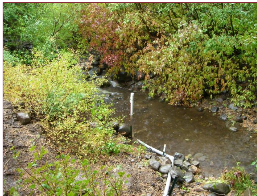
Stream flow and turbidity monitoring gauge installed in Homewood Creek.
