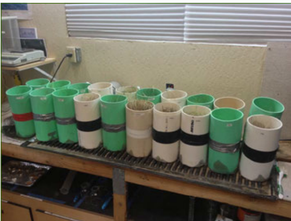
Grow-out pots used to assess plant response to different soil treatments. The most effective treatments can then be tested at the project site or used to inform cost-effective full-scale implementation.
