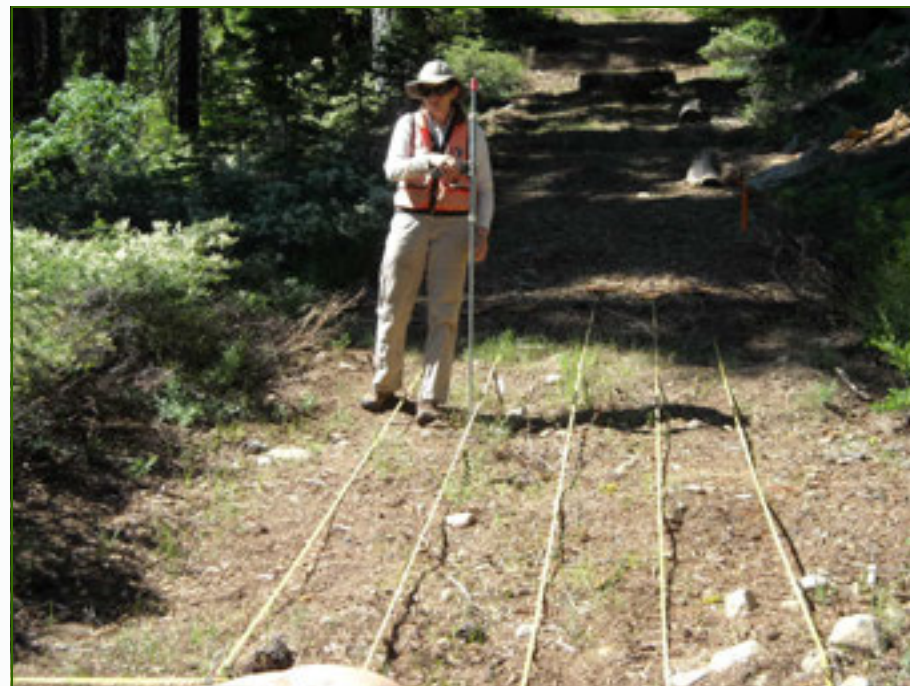
Measuring surface cover using a laser pointer along randomized transects (cover-point method).
