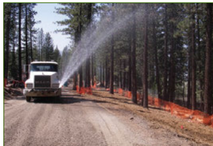
Highly adjustable fire hose nozzles (left) can be attached to water trucks to produce a wide range of spray patterns and flow rates ideal for irrigation applications. Many water trucks that are equipped for dust control applications actually displace mulch and create erosion when used for irrigation (bottom).
