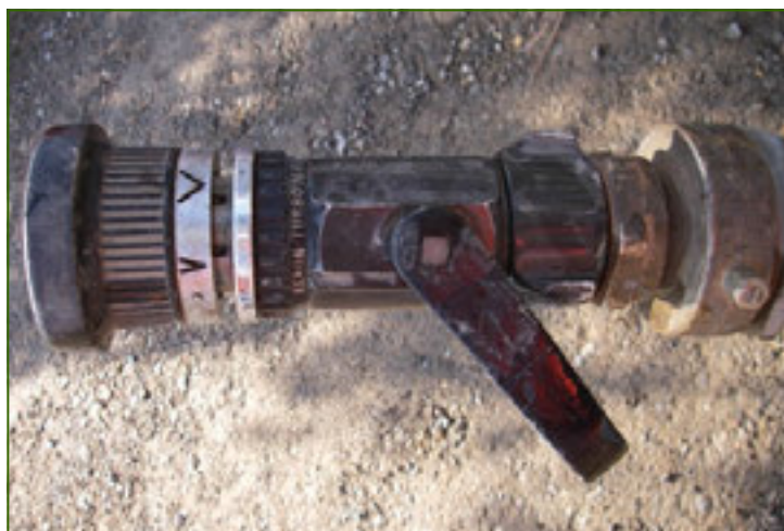
Highly adjustable fire hose nozzles (left) can be attached to water trucks to produce a wide range of spray patterns and flow rates ideal for irrigation applications. Many water trucks that are equipped for dust control applications actually displace mulch and create erosion when used for irrigation (bottom).
