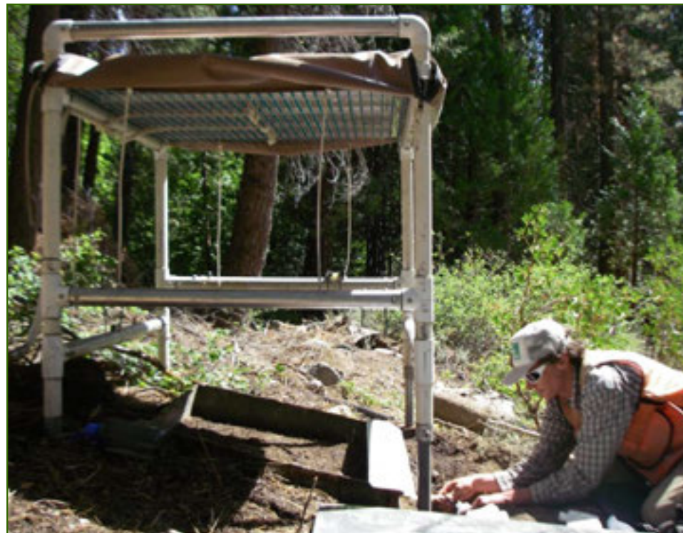
Rainfall simulation is a powerful tool for directly assessing soil hydrologic conditions.
